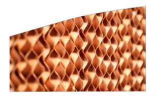
Table cooling pads are formed of grooved cellulose layers collecting reversely with its "beehive" structure forming the airflow in the cell. These layers have high capacity of water suction. They are subject to treatment with chemically odorless substance so as to prevent decomposition and provide extraordinary wetting properties, airflow, high efficiency and maximum durability.
